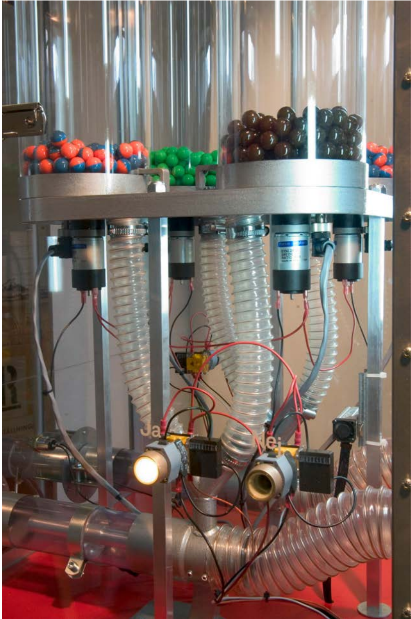
Pneumatic dispatch system for 10 av 9 är normal [10 of 9 are normal], a travelling exhibition about statistics. Visitors shoot balls and create new statistics. Photo: Riksställningar.
