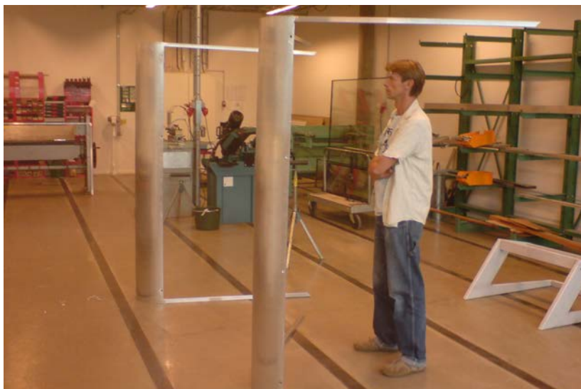
Aluminium constructions coupled with sandwich elements with a core of polystyrene between MDF for the exhibition Rewrite the Future . Photo: Mathias Strömer.
