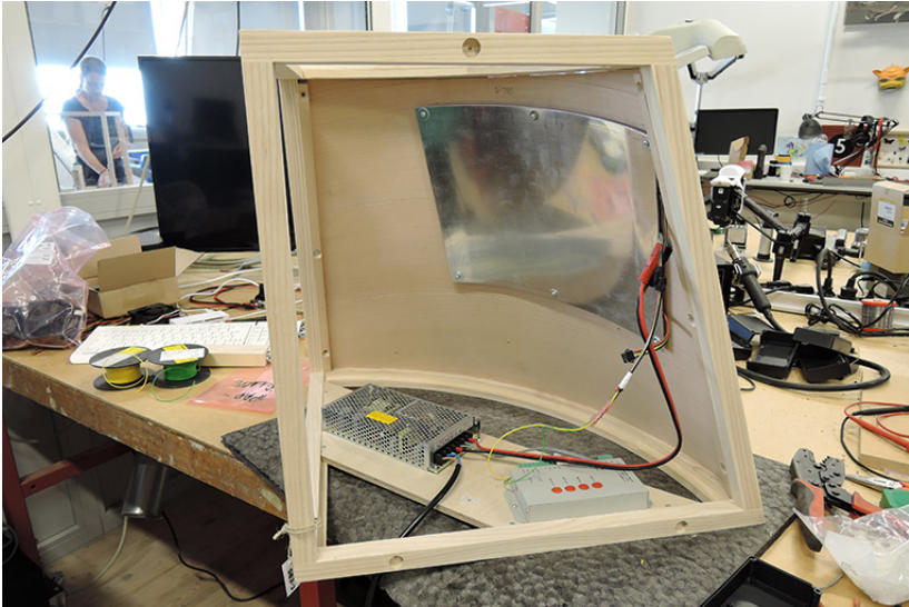
A flexible LED matrix is located behind a vaulted perforated sheet of thermo-formed plywood. The matrix is governed by a media player and is driven by a generous power supply. The intensity of the matrix means that it can be used in full daylight. Photo: Riksställningar.
