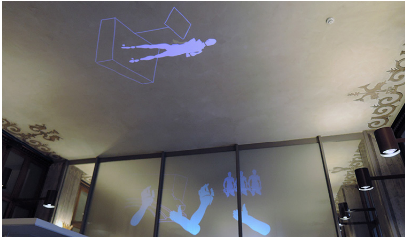
Art video projected onto a white ceiling and, using back projection, onto semi-transparent matt vinyl foil mounted on glass windows. The foil can be removed without harming the surface. Photo: Per Björklund.
