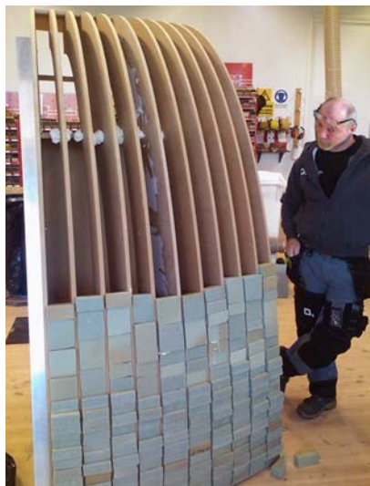
Formwork for use in casting walls. Photo: Riksställningar.
